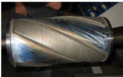
Stabilizers and other complex shapes can be addressed by precision CNC equipment
